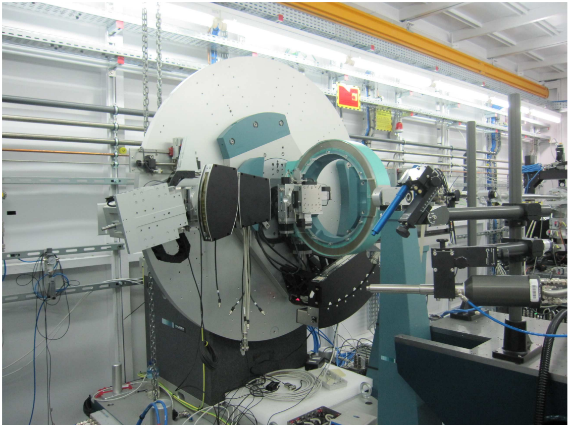
Figure 1. BL04-MSPD: Powder diffraction end station photograph. The Mythen and MAD26 detectors can be seen in the photo.
