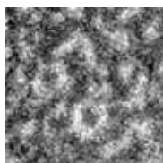
Figure 2. BL24-CIRCE: XMCD-PEEM on the Co L3 edge for an ultrathin Co film (Si/SiO/Pt(3nm)/Co(1.5nm)/AlOx).
